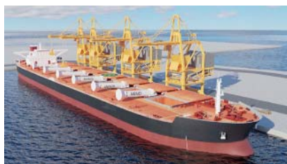
Rotors folded down to permit docking and loading of the bulk carrier (Oldendorff)
