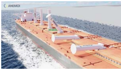
Concept of the deployment of the rotors (Anemoui)
