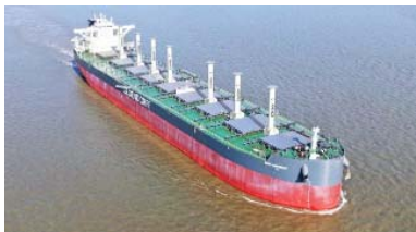
Concept of how the rotors would look installed and deployed (Oldendorff)
